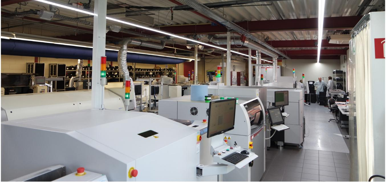
That is correct. At this stage, we really need an SPI, because we want to invest in quality and good process control. You can do this monitoring at the front of the line or at the end of the line, we choose to do it at the front.
